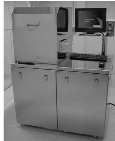
(b) NX-2000: thermal NIL and photo-curable NIL without alignment
